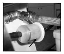
Figure 38: Secondary Fuel Filter
